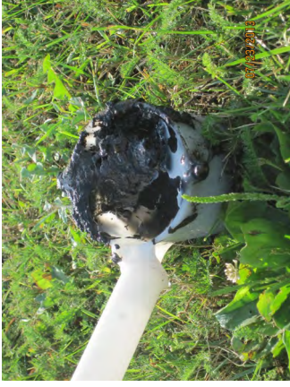
Effluent from a malfunctioning aeration system
